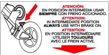
It is achieved by activating the intermediate position lever (red) located on the right-hand side of the stretcher. This releases the front legs up to a mechanical stop.
